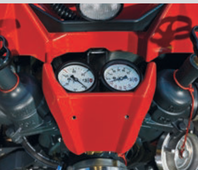
Clear and safe arrangement of pressure gauges
