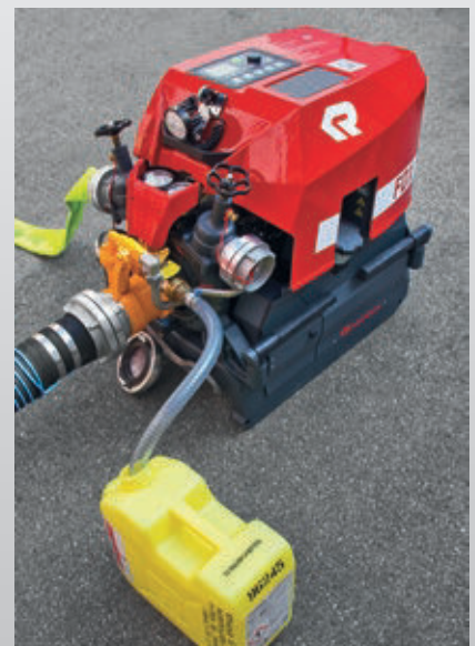
FOX with integrated foam proportioning system
